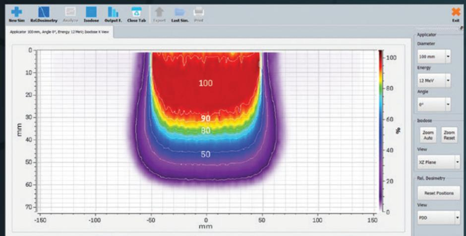
Isodose curve, applicator  $\varnothing$  10 cm, 12 MeV energy,  $0^\circ$  bevel angle.
