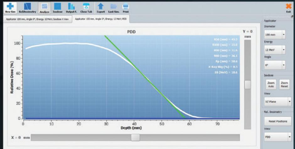
PDD analysis, applicator  $\varnothing$  10 cm, 12 MeV energy,  $0^\circ$  bevel angle.
