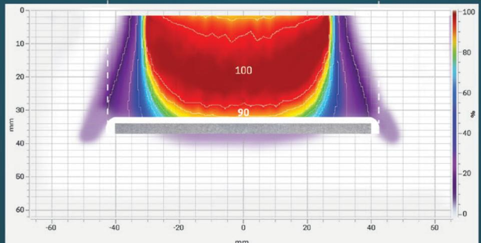
Isodose curve modified by RP disc Ø 8 cm, applicator Ø 6 cm, 12 MeV, 0° bevel angle.
