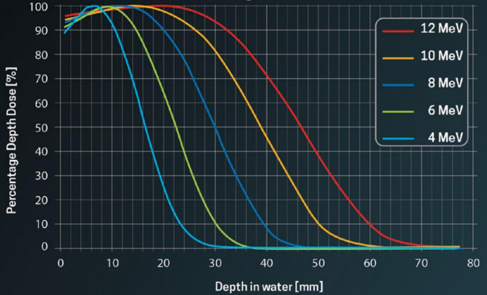
The appropriate energy and applicator selection allow to treat the target with a thickness of up to 3.8 cm inside the 80% isodose (up to 3.2 cm inside the 90% isodose).
