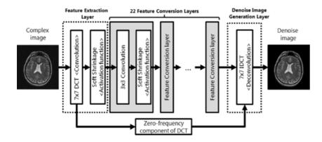
DLR is implemented after converting k-space to realspace with inverse FFT (fast Fourier Transform). After DLR processing, the rest of the reconstruction process such as zero padding zooming, gradient distortion correction and so on is done to get a final reconstructed image.
